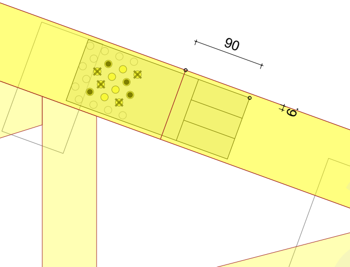
GNT150S-K 84x221 Nail: 4 no. RINGED NAIL 4 X 35 / side
