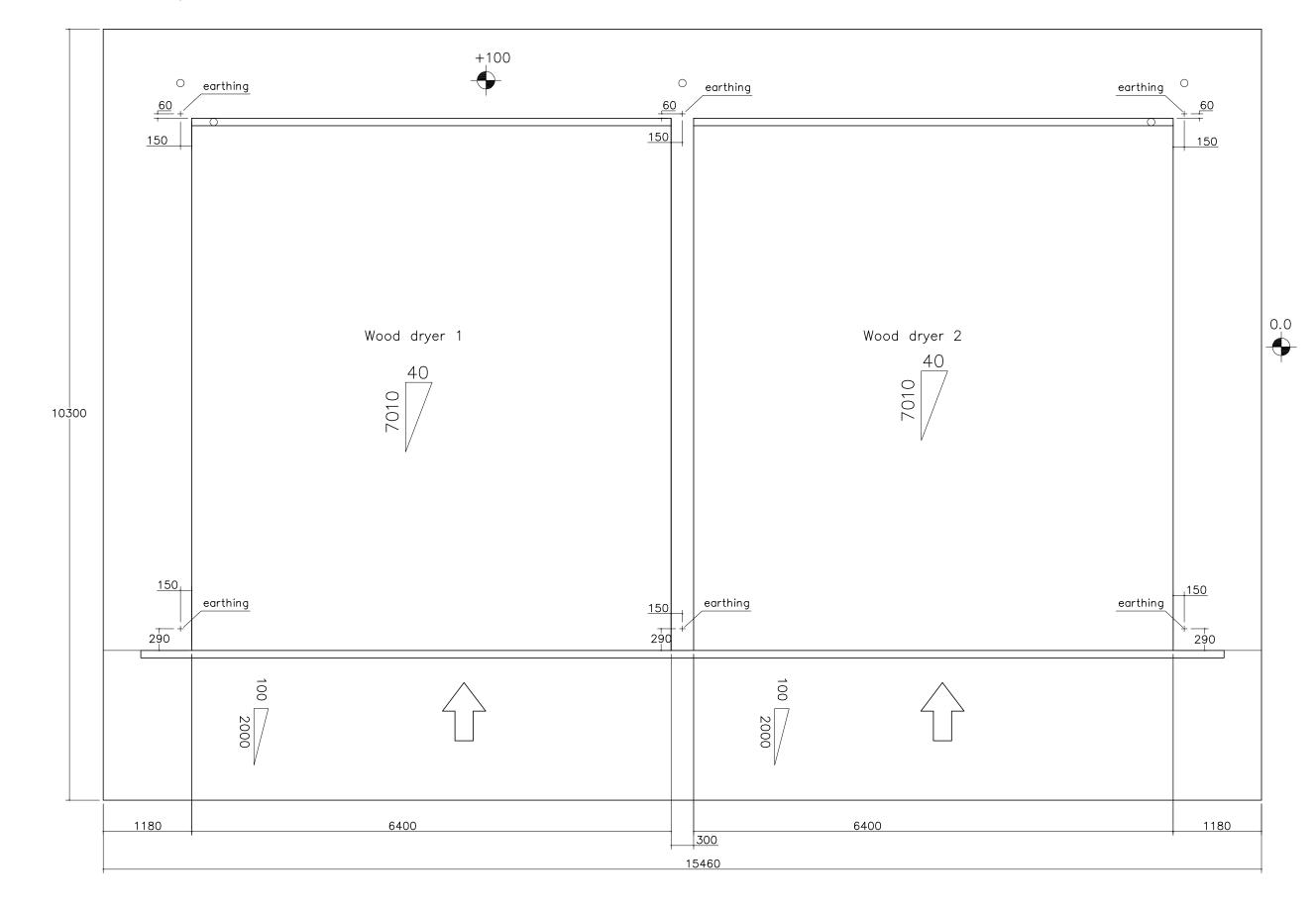
DOOR SIDE The arrows indicate the columns which are to be connected to the electrowelded NET. WARNING: the non-observance of these instructions could cause serious problems to the reading and/or precision of the wood probes. SIDE SECTION OF A PLANT WITH EARTHING connect the stainless steel square profile 100x50x3 to the still net Copper stakes Cable or copper flat for connecting the columns to the nets
